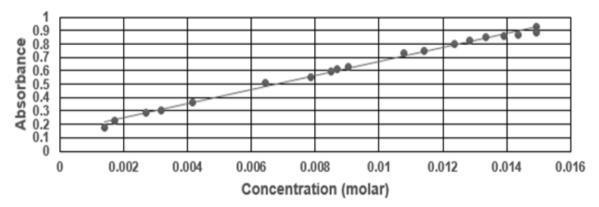
Fig. 3: Standard curve for ciprofloxacin assay. Equation of line is:  $y = 52.388 \text{ L m}^{-1} \text{ x} + 0.1435$ . The Pearson r correlation is 0.9971, with coefficient of determination  $R^2$  is 0.9943. Range of concentration is 1.3919 x  $10^{-3}$  molar to 1.4934 x  $10^{-2}$  molar.
