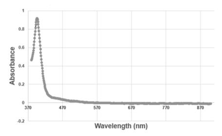
Fig. 2: The absorbance spectrum of ciprofloxacin from 380 nm to 900 nm. Ciprofloxacin at  $1.6576 \times 10^{-2}$  molar in solvent with 1% (v/v) ethanol, 98% (v/v) distilled water, and 0.167 molar acetic acid (1% v/v). Absorbance peak is located at 390 nm.
