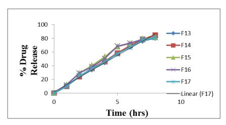
Fig. 7: In-vitro percentage drug release of ethosomes prepared by different concentrations of ethanol.
