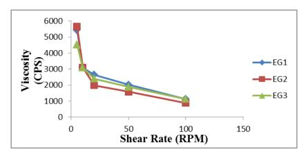
Fig. 10: Viscosity of Ethosomal gel Formulations EG-1 to EG-3.
