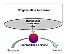
Fig. 6: Schematic diagram of a third generation biosensor.
