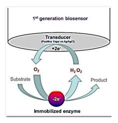
Fig. 4: Schematic representation of a first generation biosensor,
