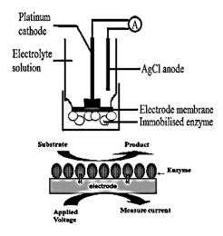
Fig. 3: Schematic representation of amperometric biosensors.
