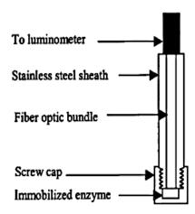
Fig. 6: Schematic diagram of an optical biosensor.
