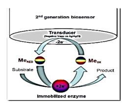
Fig. 5: Schematic diagram of a second generation biosensor.
