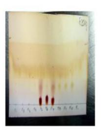
Figure 3: Thin layer chromatography of mixtures of aminophospholipids (AP1-AP3) of erythrocyte membrane with glucose or ketone bodies in the presence or absence of Larginine or creatine (Day 0, Left and Day 61, Right, F1-F10 = Vial 1-Vial 10).
