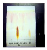
Figure 2: Thin layer chromatography of L-arginine (L-Arg) and creatine (Cr) ( $4\mu g$  /  $4\mu L$ ) dissolved in 0.1 M phosphate buffer pH 7.4. A sample of the mixture of aminophospholipids containing L-Arginine and glucose was run simultaneously for comparative purposes (Day 0).
