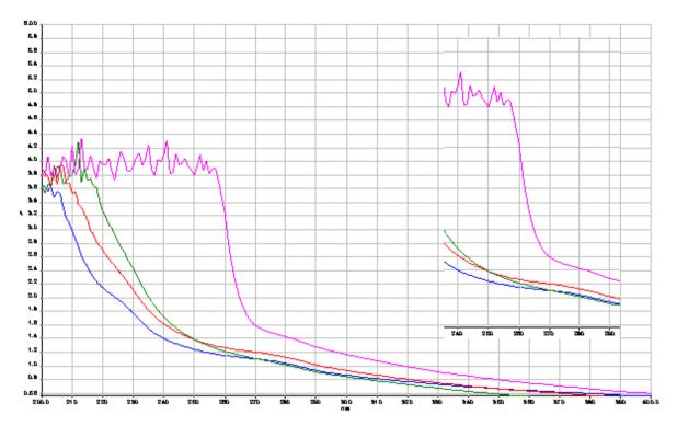
Figure 5: Aminophospholipids incubated for 61 days with glucose and L-arginine or creatine (Insert: 290-240 nm). Color blue: Vial 1. Aminophospholipids (Control). Red color: Vial 2. Aminophospholipids + Glucose. Green color: Vial 5. Aminophospholipids + Glucose + L-arginine. Pink color: Vial 8. Aminophospholipids + glucose + creatine. Absorbance vs.  $\lambda$  (nm).
