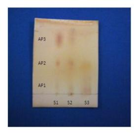
Figure 1: Thin layer chromatography of aminophospholipids (AP1-AP3) obtained from human erythrocyte membranes. In each plate the samples were applied in triplicate (S1-S3).
