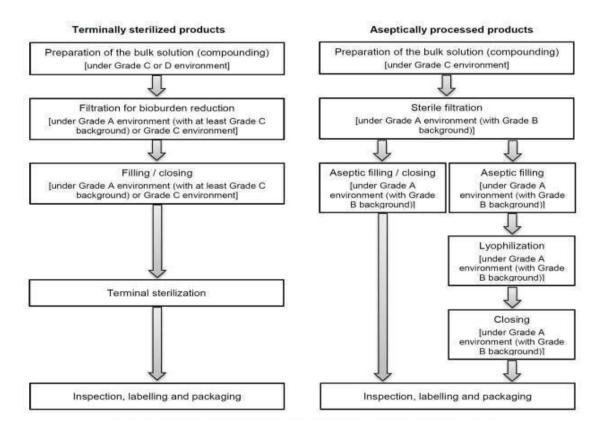
Figure 2: General steps involved in the manufacture of injectable drug products.
