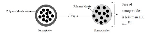
Fig. 3: Nanospheres and Nanocapsules.
