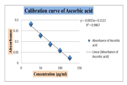
Graph 3: Calibration curve of Ascorbic acid.
