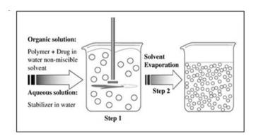
Fig. 10: Schematic representation of solvent evaporation technique.
