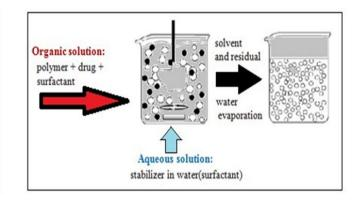
Fig. 13: Schematic representation of Nanoprecipitation technique.
