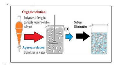
Fig. 12: Schematic representation of emulsification /solvent diffusion technique.
