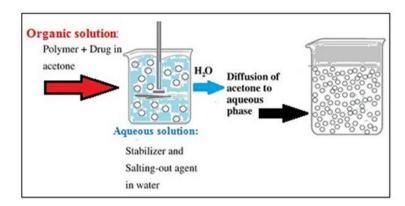
Fig. 11: Schematic representation of salting out technique.
