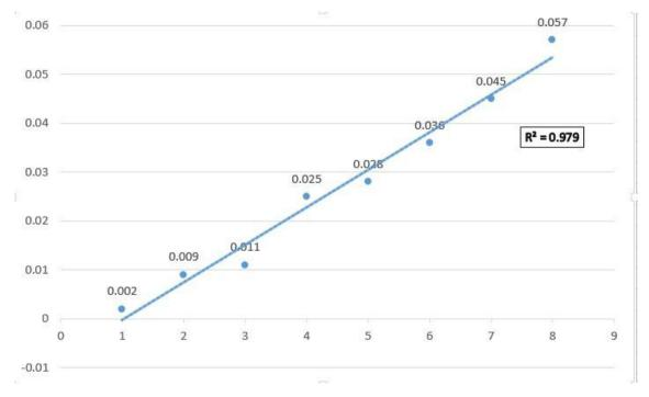
Figure 2: Standard curve of Ibuprofen Comparison of dissolution profile Dissolution test for local Ibuprofen 400mg tablet.
