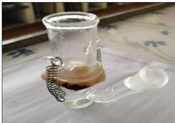
Figure 4: Working of Franz Diffusion Cell.
