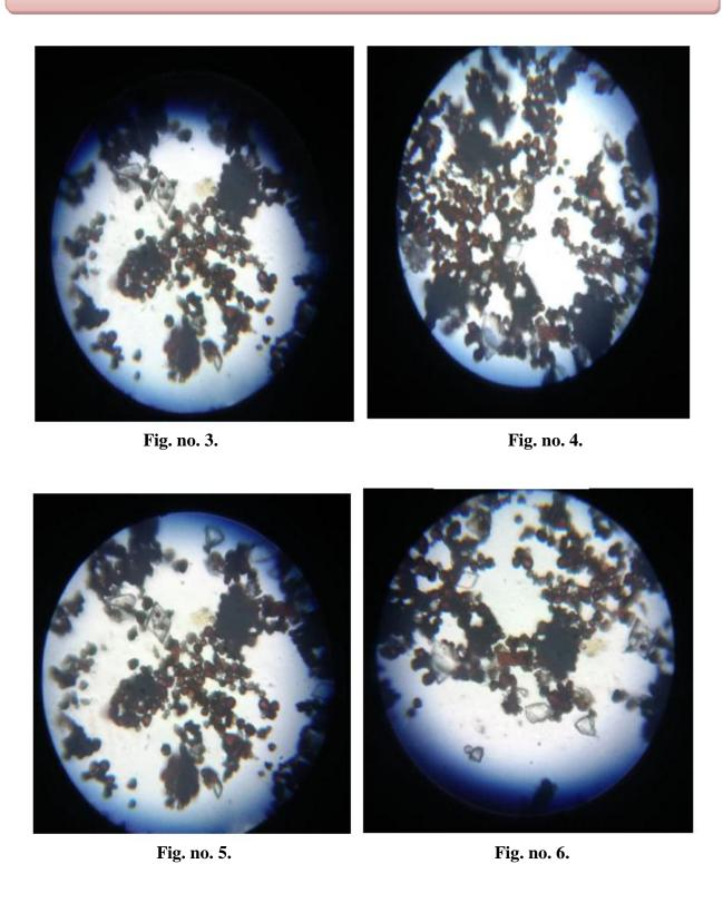
Starch grains and calcium oxalate crystals stained with Iodine solution shown in fig 3-6.
