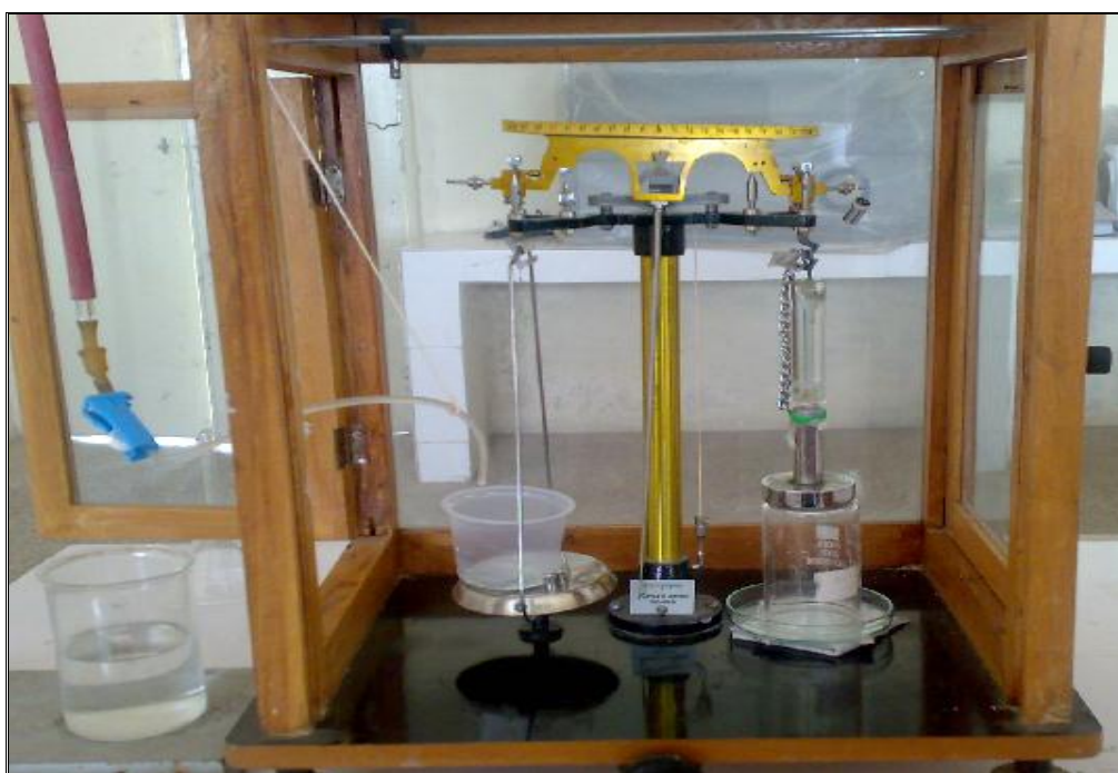
Fig. 1: Modified Mucoadhesion Test Apparatus.
