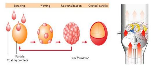
Figure No: 4 Process principle of fluid bed coater.
