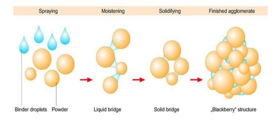
Figure No. 3 Process principle of fluid bed granulation.
