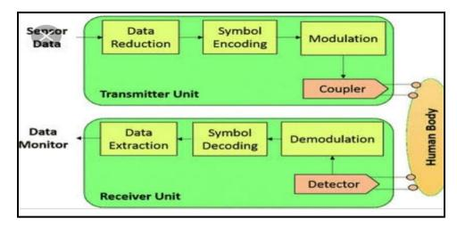
Fig. 2: In vivo communication for data transmission between sensors enabled by transmitter and receiver units.
