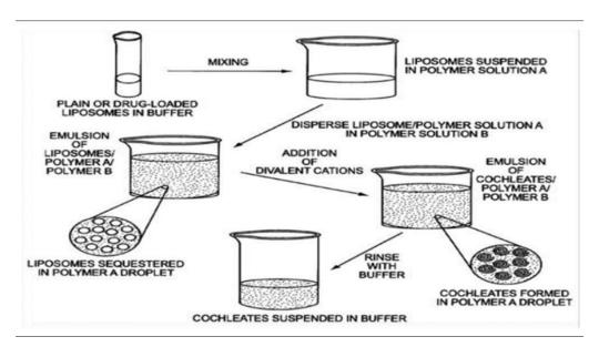
Fig. 5: Preparation of Nanocochleate by Hydrogel method. [2,33]
