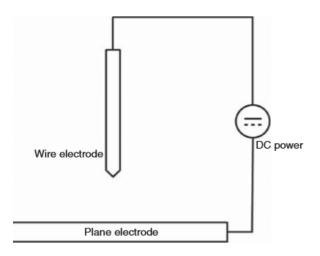
Fig. 4: Corona Discharge (Schematic Representation).
