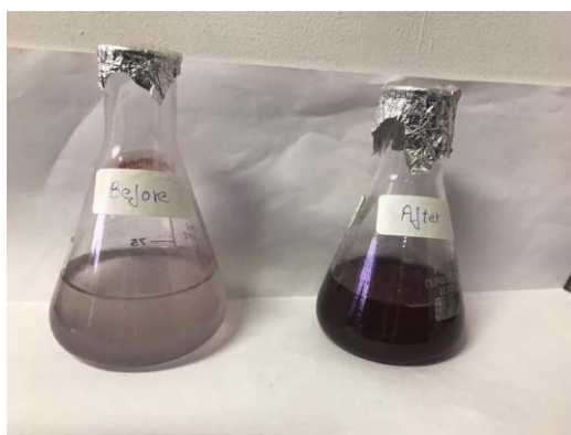
Figure 1: Colour Change indicating the formation of gold nanoparticles.
