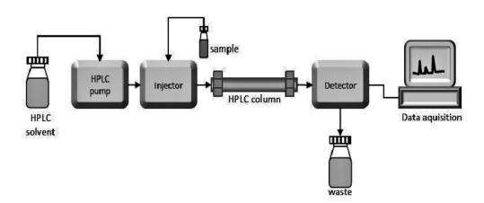
Fig. 1: Flow diagram of HPLC.
