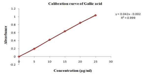
Figure 1: Graph of calibration curve of gallic acid.
