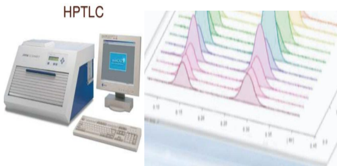
Fig 6: Densitometer and Obtained Chromatograms by Densitometer.
