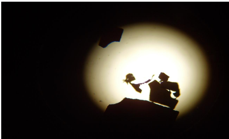
Figure 08: The hafnocene product had white fibers about 0.1 cm in length an aspect ratio of about 1000. The fibers appear to hold the flat plates together.
