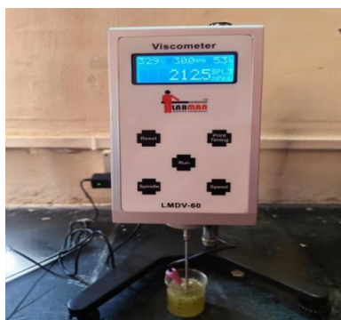
Fig.0.6: Viscosity determination by the Brookfield Viscometer.
