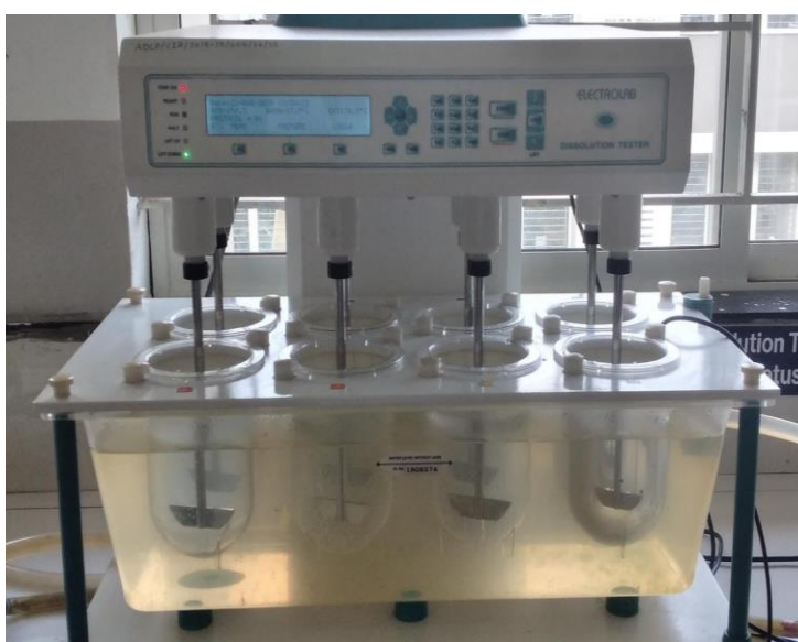
Figure No.1.19: Instrument of Dissolution Apparatus.
