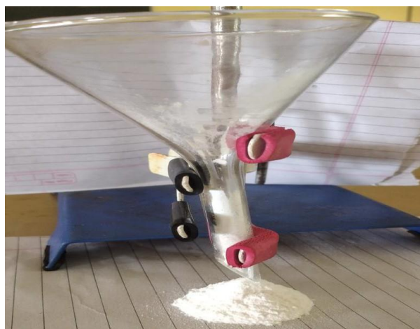
Figure No. 1.5: Apparatus of Angle of Repose.
