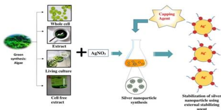
Figure 3: Green chemistry approach for synthesis of AgNPs. [36]
