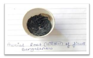
Weigh a clean, dry porcelain crucible and records its weight. Then add 2 gm of powder into crucible and record the total weight. Place in oven at 600 c for 2 hours, and then allow to cool. Weigh the crucible with ash and record its weight.
