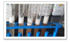
This test is performed to check the foaming ability of the formulated shampoo. Five test tubes are taken and add then add the sample to test tube in increasing order (1ml, 2ml, 3ml, 4ml,5ml), the volume of each test tube is make up to 10 ml. then the tubes are shaken and then the foam is calculated.
