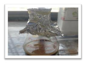
The 2 gm powder of banyan aerial roots weighed and macerated with water, ethanol with occasionally stirring. The extract is filtered to remove any solid particles. The filtrate is then evaporated to dryness and the residue is then dried.
