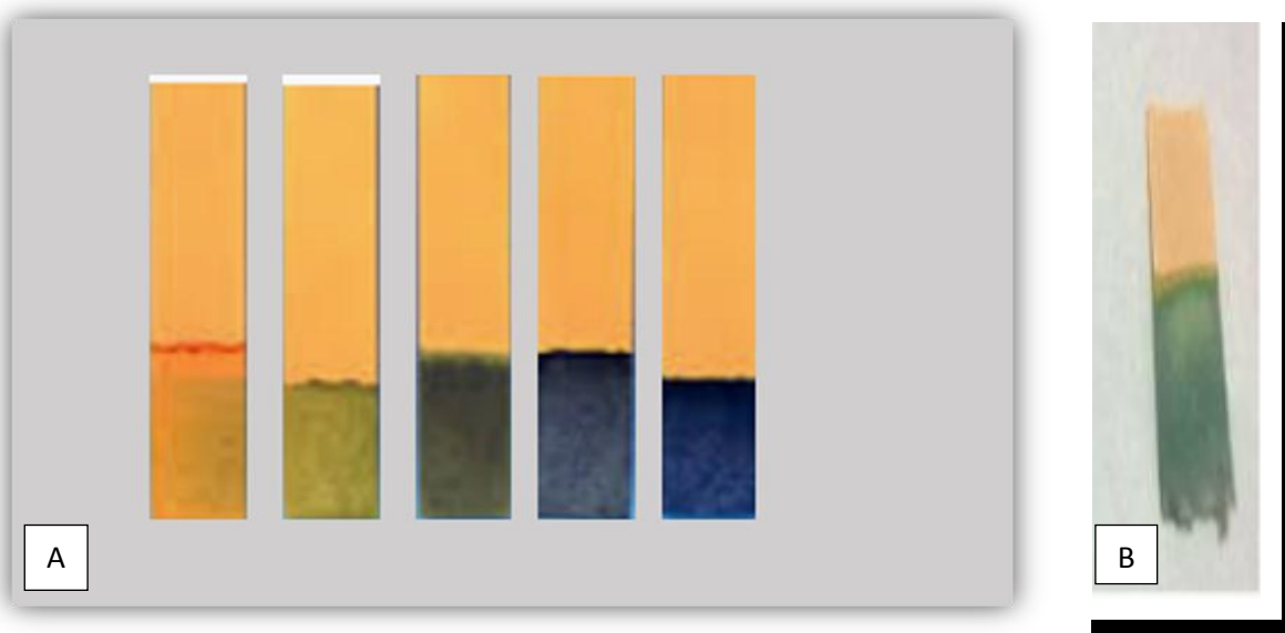
Figure 8.1. Determination of pH using pH paper strip and standard pH scale along with other standard reference materials.
