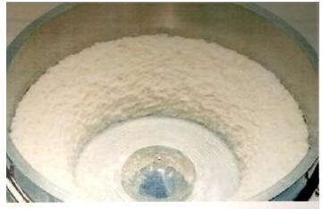
Figure.5. Process of spheronization
