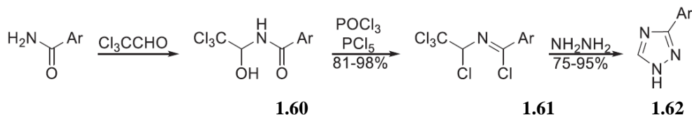
Fig. 19. Reaction scheme of the reactive N-polychloroalkyl imidoyl chlorides with hydrazine with the formation of monosubstituted 1,2,4-triazoles.
