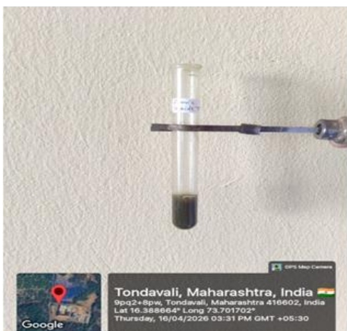
Fig. No. 13: Ferric Chloride Test For Mimo.
