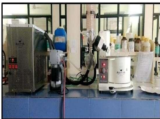
Formation of thin film using Rotary evaporator
