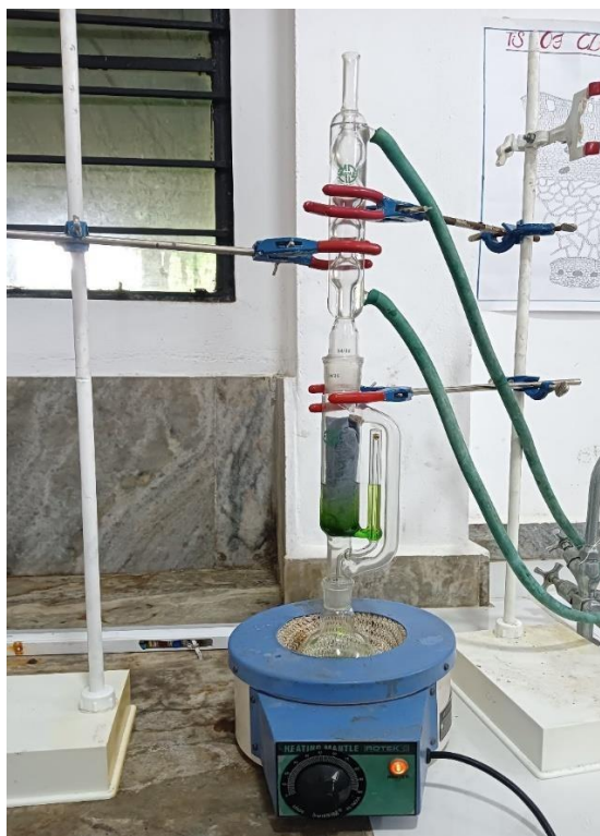
Fig. 9: Red spinach extraction by soxhlet apparatus.
