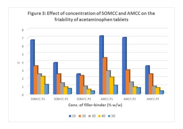
bonding capacity. At polymer concentration of 50% w/w, compact exhibited friability lower than 2% at all compression pressures above 31.2 MPa.
