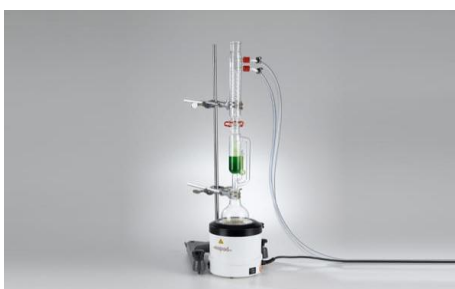
Extract preparation using Soxhlet apparatus
