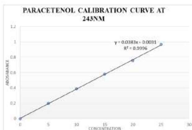
Figure 3: Calibration curve of Paracetamol in Distill water (Linearity of paracetamol).
