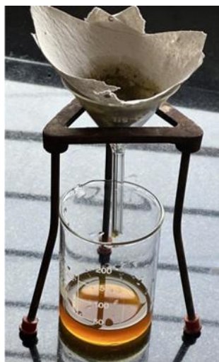
Figure 3: Maceration and filtration of licorice extract.
