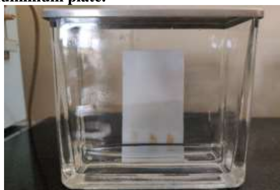
Figure 17,18: Developing Chamber with Toluene: Ethyl acetate: Formic acid: Methanol Solvent System.
