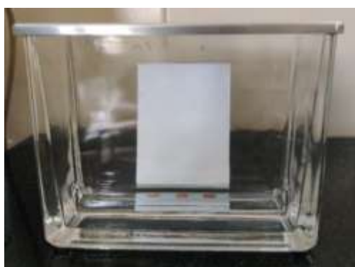
Figure 17,18: Developing Chamber with Toluene: Ethyl acetate: Formic acid: Methanol Solvent System.
