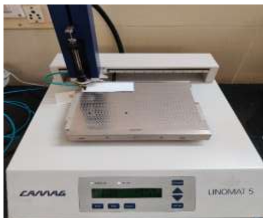
Figure 15: Sample application on a pre-coated silica gel F 254 on aluminium plate.
