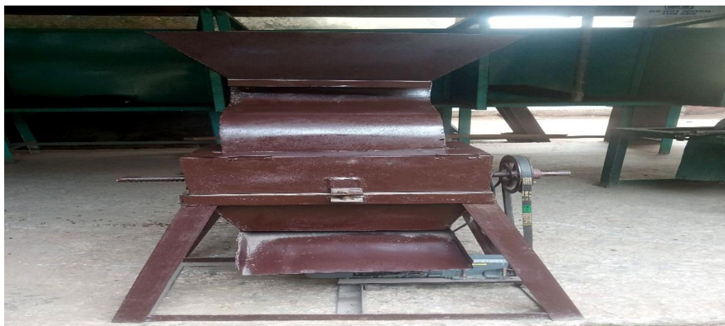
Figure 1: fabricated breadfruit dehuller (dimensions 450 x 250 x 750 mm 3 ).
