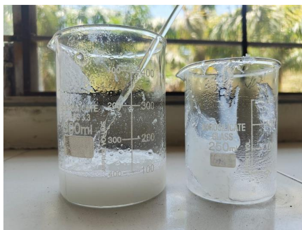
Fig. 4: Carbopol & HPMC base gel preparation.
