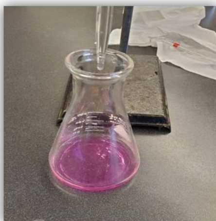
Fig no. 16: determination of Acid Value.
