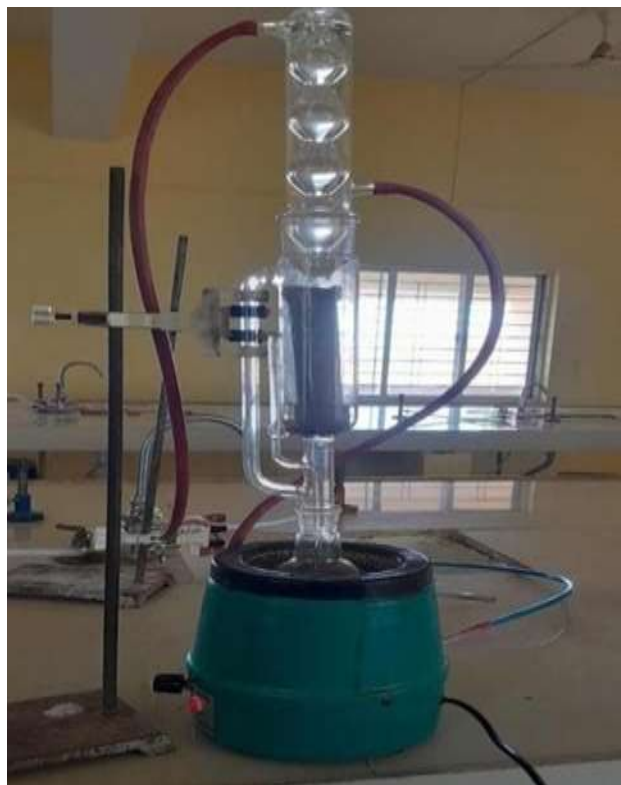
Fig. 9: Extraction of Cucurbita oil.
