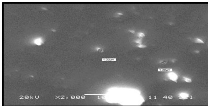
Fig. 1: SEM image for 30:1 ratio silver nanoparticles.
