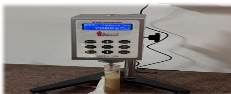
Fig No:1 Viscosity determination by Brookfield viscometer.
