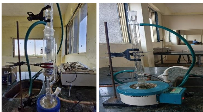
Figure 6: Soxhlet Extraction of Mahua and Soxhlet Extraction of Adulsa.
