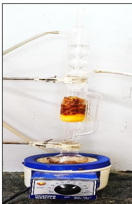
Figure 1: Soxhlet extraction of Test sample (CI).
