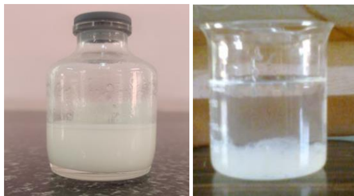
Figure 5: Conversion of sol to gel.
