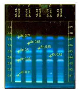
(Image AT 366nm, After Development, seven Strong flurocence band was observed at RF: 0.11,0.35,0.42,0.50,0.55,0.63,0.74)
