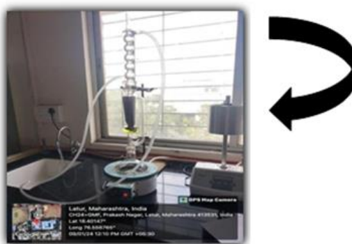
Image No. 3: Extraction of Ficus racemosa fruit powder by Soxhlet Apparatus
