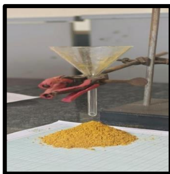
Fig 3: Determination of Angle of Repose.
