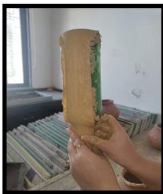
Fig. 5: Layering of cloth on kupi.
