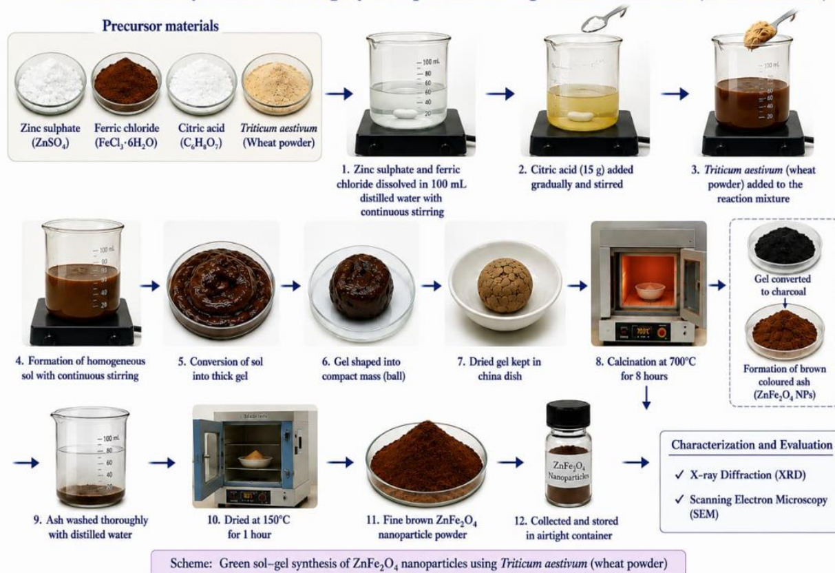
Figure 4: Experimental Procedure for the Green Sol–Gel Synthesis of Zinc Ferrite ( \text{ZnFe}_2\text{O}_4 ) Nanoparticles.
